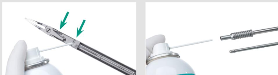
For smooth running of the instrument, lubricate all moving parts and joints of the shaft with a steam-permeable lubricant (e.g. Aesculap STERILIT® I oil spray JG600). After lubrication of the shaft please open and close the jaw part several times by pushing the lever and handle.
