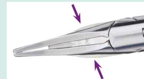
**B:** Hold the edges of the clip cartridge with your thumb and index finger and pull the cartridge off from the applicator shaft.
