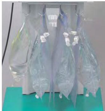
Fig. 4-7 Bags on load cell
